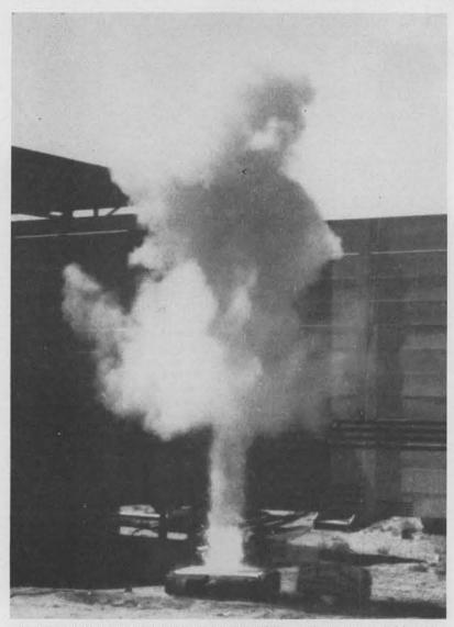
MINIATURE BLAST assumes the familiar shape of a mushroom cloud as a half-ounce charge of high explosive is exploded in Area III. The laboratory-scaled model blast is one of the series in an exploratory study to determine cratering effects of explosions.
